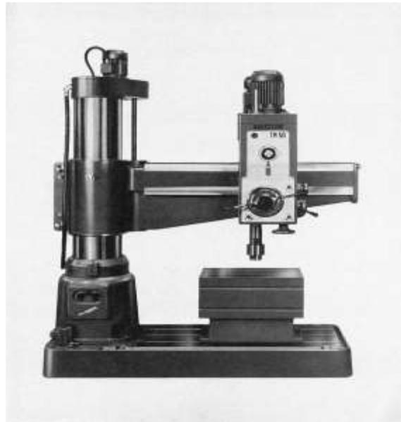
FIGURE 9.11 Radial drill press.
