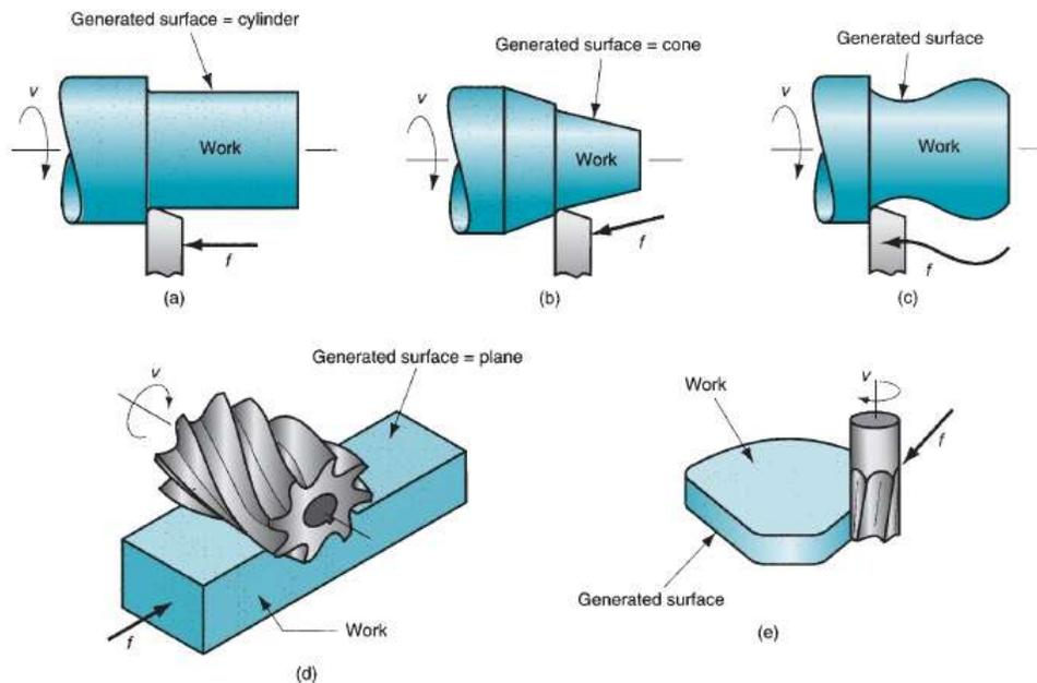
FIGURE 9.2 Generating shape in machining: (a) straight turning, (b) taper turning, (c) contour turning, (d) plain milling, and (e) profile milling.
