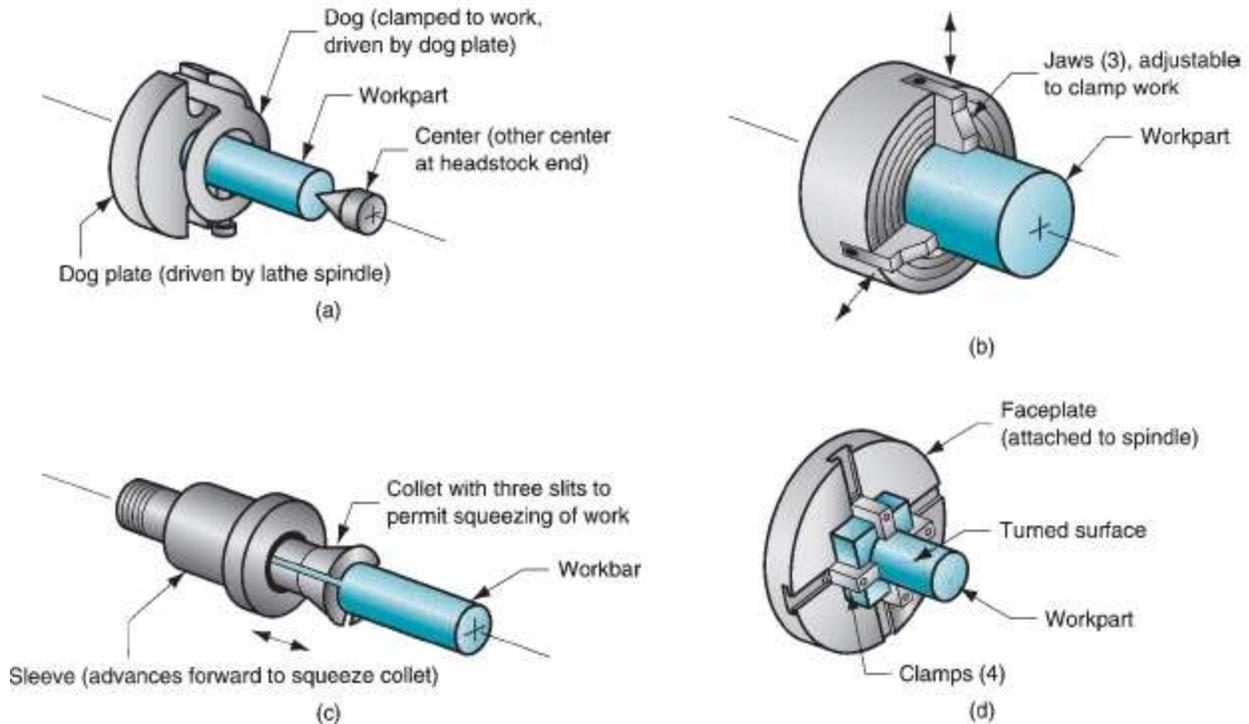
FIGURE 9.8 Four workholding methods used in lathes: (a) mounting the work between centers using a dog, (b) three-jaw chuck, (c) collet, and (d) faceplate for non-cylindrical workparts.
