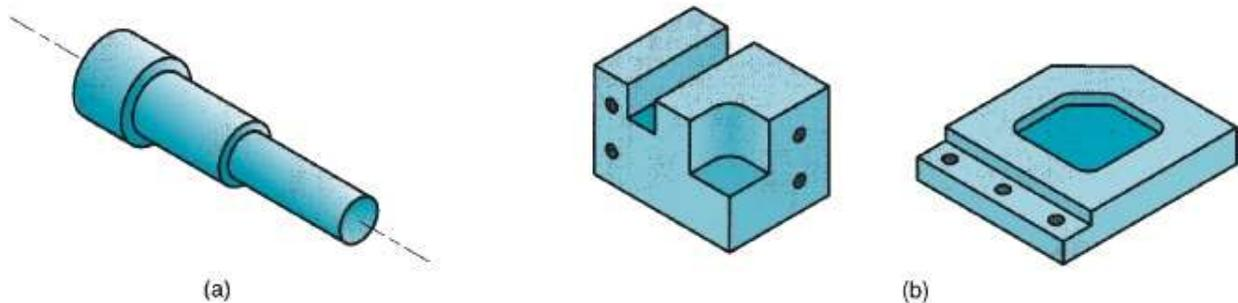
FIGURE 9.1 Machined parts are classified as (a) rotational, or (b) nonrotational, shown here by block and flat parts.
