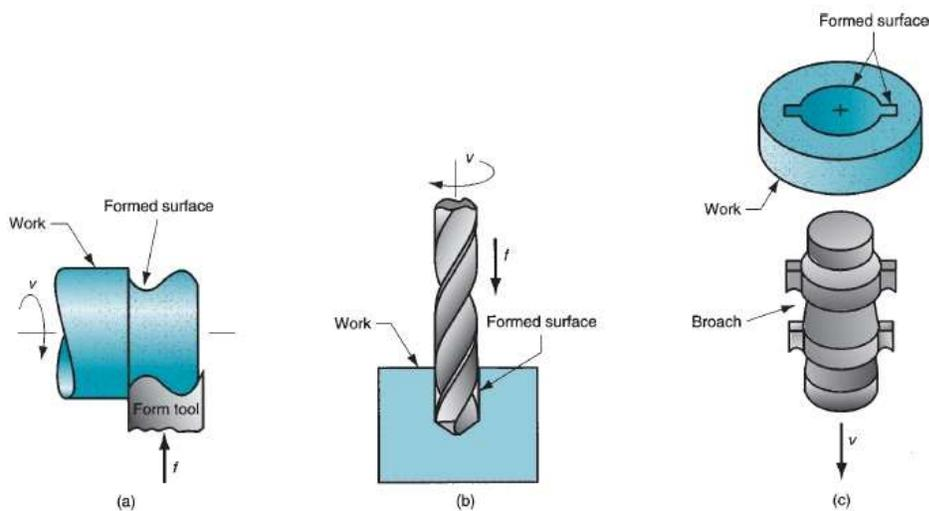
FIGURE 9.3 Forming to create shape in machining: (a) form turning, (b) drilling, and (c) broaching.
